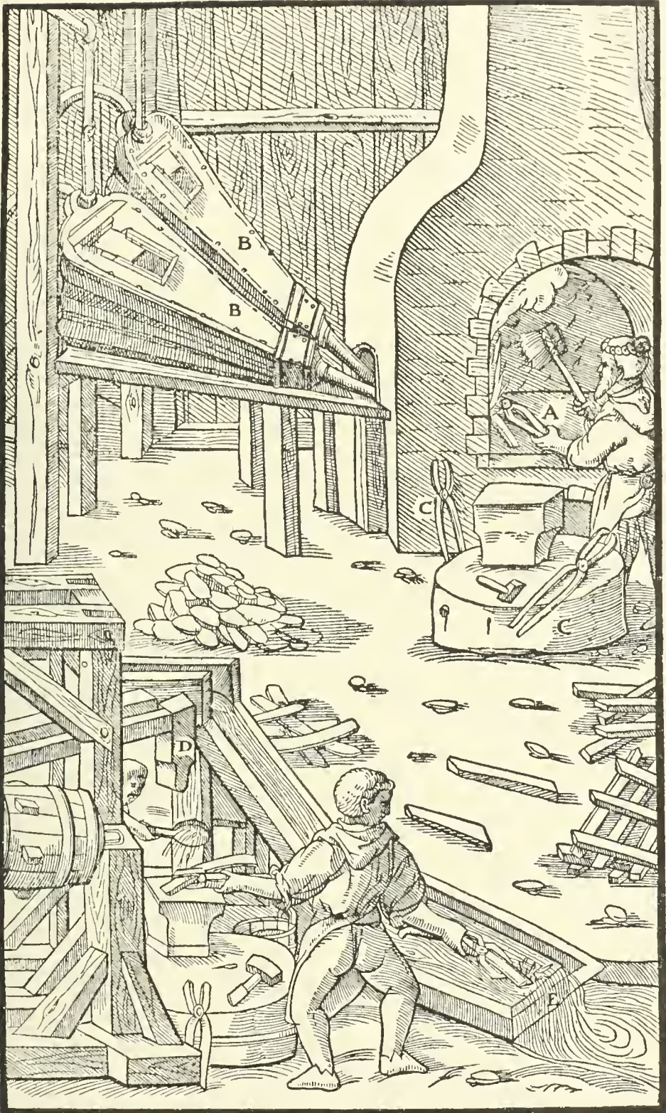
A—FORGE. B—BELLOWS. C—TONGS. D—HAMMER. E—COLD STREAM.
